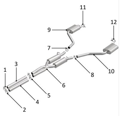
**STEP 1:** (Carefully read all instructions before installation) Disconnect the vehicle's battery before removal of the OEM exhaust system. This will prevent electrical accidents and will reset the computer if it applies to the vehicle. Remove existing exhaust system from the vehicle. Only remove parts that will be replaced. Clean existing flange with a wire brush to ensure proper sealing.
